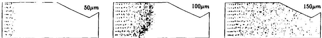
Figure 9. Spray parcel distribution for three initial spray conditions ( \phi = 1.3 , C_{pert} = 0.02 , E_1 )
